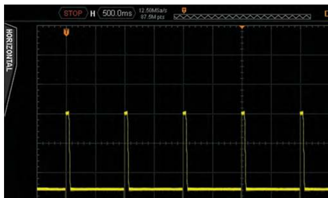
DC Voltage Transient Output Captured
