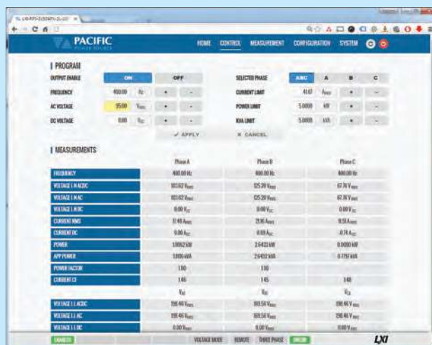
Control and Measurements Page shows settings and read backs
