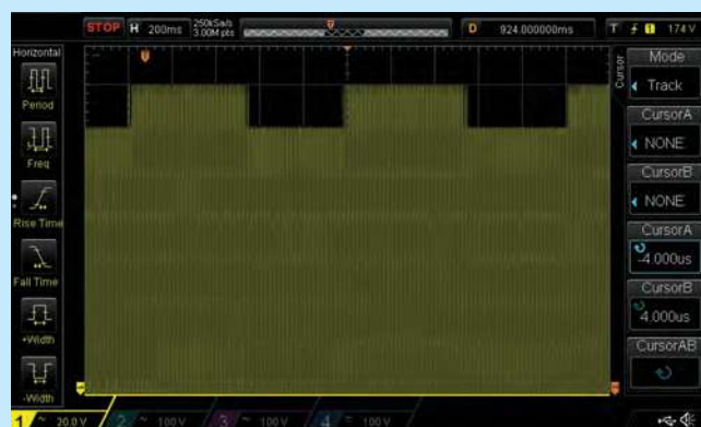
Voltage Modulation Test @ 1Hz Captured
